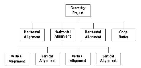
InRoads provides tools to help you design the vertical geometry within AAHSTO or CDOT project guidelines. You can also create multiple vertical alignments for each horizontal alignment if you wish to analyze different alternative alignments for cut/fill balancing or other design criteria (vertical curve designs, vertical grades, stopping sight distances, etc.)
