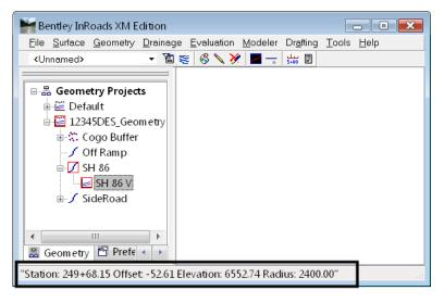
• *Tools > Tracking > Vertical Alignment* – tracks the vertical alignment on the profile grid with a vertical line to your cursor. It gives a Station, vertical Offset, Elevation and vertical alignment Grade readout at the location of your cursor.
