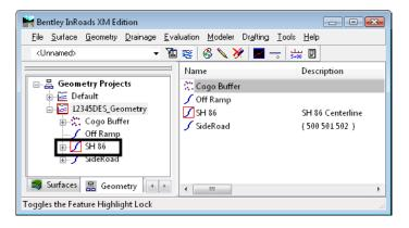
Once the geometry project is loaded (and correct horizontal is active), you may create a new alignment name using the *File > New > Geometry* command.
