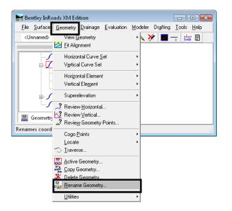
• **Rename Geometry** – to rename a vertical alignment. For example, when you are using an existing geometry project with alignments from Survey, you can use the **Rename Geometry** command to give the alignments project specific names.
